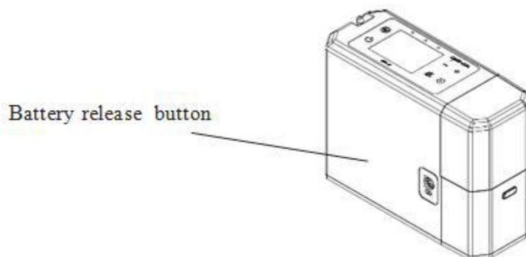
Press and hold the battery release button inward and then pull up to slide the battery pack out.
