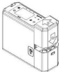
**Battery installation:** Put the battery in the slide rail, please follow direction of the arrow
