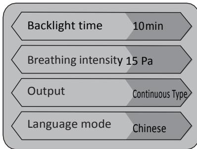
Press the setting key again to set the backlight time, breathing intensity, output mode and language selection in turn. When selecting a language option, press the setting key again to return to the main interface.
